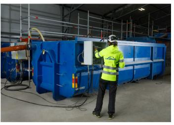
The standardized and CE-marked SOLVOCARB® dosing panels provide capacities up to 20 kg  $\rm CO_2/h$ . The gas dosage is automatically regulated towards the desired pH-value through continuous pH-measurement.
