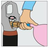
5. Pull the opening of the balloon over the rubber part of the nozzle. Push the rubber part downwards to fill the balloon. Once the balloon is almost full, finish filling carefully.
